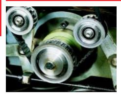
Gates classical synchronous PowerGrip® belts offer a maintenance-free and economical alternative to conventional drives like chains and gears. Applications range from minimum drives (printers) to heavy-duty machinery (oil pumps, etc).
