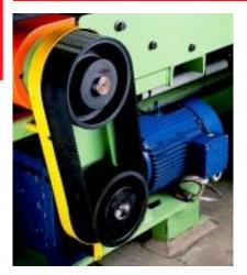
PowerGrip® HTD® drives provide positive power transmission for a wide range of industrial applications, and offer many advantages over conventional chain and gear drives.
